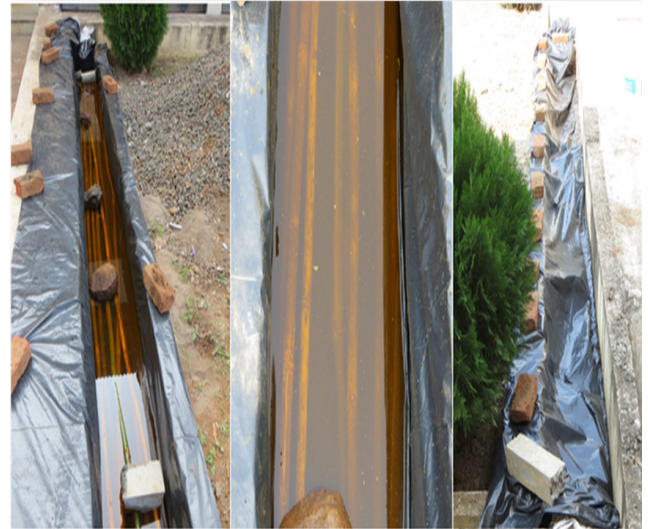
Fig.2 Bamboo Preservation by Dip Diffusion Method
